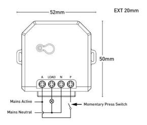
Note: A momentary press switch returns to the open position when released. If an external switch cannot be installed, leave the 'P' control terminal unconnected.
